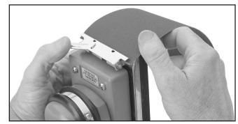
Figure 2. Attaching sanding sheet.
